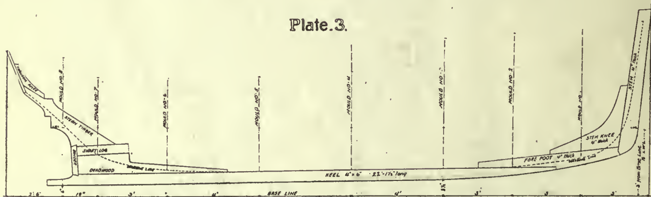
Names of the various pieces that, when all are bolted together, form the backbone of the boat's frame and the location for the various molds.
