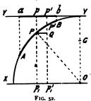
considered proportional to the length of the line, and we may therefore say that the moment of  $PP^1$  about OX is  $PP^1 \times Pp_1$ ;  $Pp_1$  being drawn perpendicular to OX; and  $P^1Q$  being negligible compared with  $Pp_2$ .
