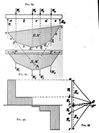
new link-polygon (fig. 89) be drawn. If a thin wire be made to the same outline as this same polygon and be attached to the beam, and the loads  $W_1$ ,  $W_2$ ... attached at the angles, it is evident that the compound structure formed by the bar and
