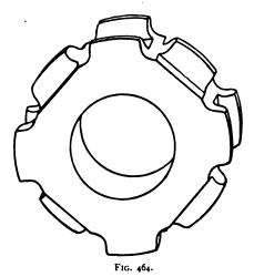
have the form shown in figure 464, in which the alternate teeth are in duplicate at the edges of the rim. For tandems. triplets, &c., a still greater pitch, say 11 inches, may be used with advantage : the back-hub chainwheel, with six teeth of this pitch, would have the same average radius of pitch-polygon as a chain-wheel with nine teeth of  $\tau$  inch pitch; the chain would have only one-third the num-
