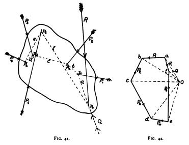
cutting the line *a*, the line of action of the added force Q, at  $p_r$ . The resultant of Of and -Q is af = R (fig. 42), and it acts through the point  $p_r$ .
