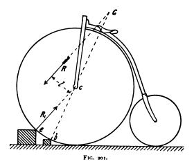
ference of the wheel at b. A stone touching the rim at a point higher than b may cause a header at high speed; a stone touching at a lower point may be ridden over at any speed. Figure 200 is the same diagram for a 'Safety' bicycle, a glance at which shows that with this machine a much larger stone can be safely surmounted than with an 'Ordinary.'
