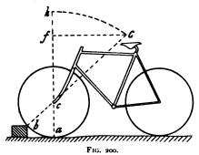
supplied by the action of the ground on the wheel. is transmitted This the wheel. through so that an equal force,  $F_2$ , acts on the mass at G, and the mass reacts on the frame with an equal and opposite force,  $F_{a}$ . Then, in order that stability may be maintained, the resultant R
