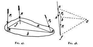
third side a b of the force triangle. Comparing with figures 41 and 42, the truth of the above construction is obvious.
