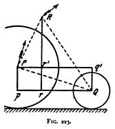
in directions at right angles to QP and QR respectively, and their speeds will be  $\omega \times QP$  and  $\omega \times QR$  respectively; the lines QPand QR (fig. 223) may therefore represent the magnitudes of the velocities, the directions being at right angles to these lines. Through Q draw a horizontal line, and to it draw perpendiculars Pp and Rr. Then Qp and Qr will represent the vertical components of the motions of P and Q respectively, Pp and Rrthe horizontal components.
