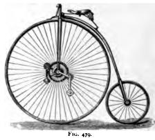
crank is  $\frac{N_1 + N_3}{N_1}$ . If the driving-wheel be 40 in. diameter, and the pinion and hub have 10 and 30 teeth respectively, the bicycle is geared to  $\frac{30 \times 10}{30}$   $\times$  40 in. == 53.3 inches. It should be noticed
