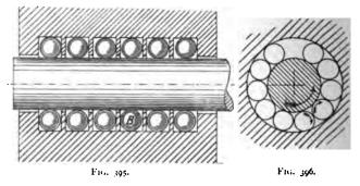
this case would be that each ball would have contact with the shaft and the bearing-case at a *point*, while each cylindrical roller had contact along a *line*. As a matter of fact, the surface of contact in the case of the ball-bearing would be a circle of very small diameter (point contact), while in the case of the roller-bearing it would be a very small, narrow rectangle of length equal to that
