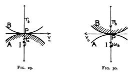
evidently coincide with the centre of curvature of the body A at the point P; then  $U_a$ , the rubbing of B on A, takes place with speed,  $V_a = \omega r_a$ , and is therefore equivalent to a translation  $V_a$  and a rotation  $\frac{V_a}{r_a}$ , or
