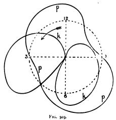
Geared Facile.—Figure 502 shows the polar curves of pedal speed, p p, and of speed of knee-joint, k k, for a Geared Facile :
