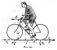
the acceleration, the frame must act on the mass, and the mass react on the frame with an equal but opposite force, f. Introduce at the point of contact of the driving-wheel with the ground two equal and opposite forces,  $f_1$ and  $f_2$  (fig. 191), each equal and parallel to f; then f is equivalent to the force  $f_1$ , and the couple
