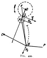
relative to the frame, but the speed of the crank is not constant, on account of the oscillation of the coupling-rod and planet-wheel.
