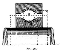
as the front axle of an 'Ordinary,' tricycle axles, &c. This bearing supports the load at right angles to the axle and at the same time resists end-way motion. A ball has contact with the ball-races at four points, a, b, c, d, which for the best arrangement should be in pairs parallel to the axis; the motion of
