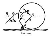
moving with velocity v in a norizontal direction. This can be resolved into a velocity  $v_1$  in the direction  $c_1 S$ , joining the wheel centre to the stone, and a velocity  $v_2$  at right angles to this direction. The velocity,  $v_1$ , is the velocity of impact of the wheel on the stone S, and the energy due to this velocity may be entirely lost.
