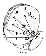
axis *Pd* lying in the tangent plane. relative motion of two bodies in contact is compounded of 'rubbing,' 'rolling,' and 'spinning.'
