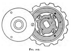
the balls,  $\delta$ , were liberated, and the cog-wheel revolved quite independently of the axle. While moving in a straight line both driving-wheels were driven; but when running in a curve the inner wheel was driven by the clutch, while the outer wheel running faster than the inner overran the axle and liberated the balls, the outer wheel being thus left quite free to revolve at the required speed.
