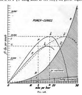
to overcome air resistance is TR; and the total power required is the ordinate SR. The curve M can be lowered by improvements in the mechanism, the curve T by improvements in the tyres and track-surface, and the curve R by improvements in pace-making.
