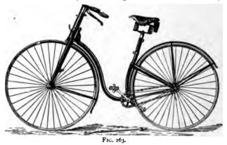
tube is subjected to a bending stress, while the frame, as a whole, is weakest in the neighbourhood of the crank-axle. Since the bending-moment on the frame diminishes from the crank-axle
