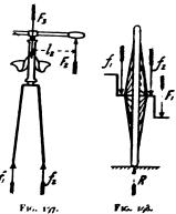
Now, consider the forces acting on the wheel (fig. 198), including cranks and pedal-pin, which together form one rigid body. Besides the forces  $F_1$ ,  $f_1$ , and  $f_2$ , there is only the reaction of the ground, R, and since the wheel is in equilibrium vertically,
