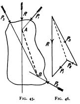
of the link-polygon, cutting the side  $P_1$  of the force triangle at b. The force  $P_2$  is represented in magnitude and direction by the
