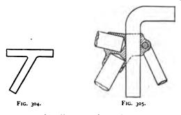
the stresses due to bending; or, for a given range of horizontal adjustment, the bending stresses are lower with the T-shaped than with the L-shaped seat-pillar. The adjustment got by an L pin with horizontal and vertical limbs is much better (figs. 256, 260), since by turning the L pin round, the saddle may be adjusted either before or behind the seat-lug S. Thus,
