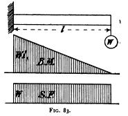
equal to W for all sections; the shearing-force diagram is, there fore, a straight line parallel to the axis.
