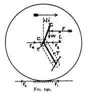
position, vertically above the axle of the wheels; the machine is thus in stable equilibrium laterally and in unstable position longitudinally. In driving along at a uniform speed against a constant wind resistance, F (neglecting at present other resistances), the mass-centre, G, is in its normal position, a short distance, l, in front of the axle (fig. 190). While the rider exerts the driving effort the wheel exerts the force  $F_1$  on the ground, directed
