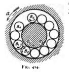
a ball-bearing properly adjusted the adjusting cone is not screwed up quite tight, but is left in such a position that the balls are not all held at the same moment between the cones and cups; in other words, there is a little play left in the bearing. Figure 414 shows such a bearing sustaining a vertical load, as in the case of the steering-wheel of a bicycle, with the play greatly exaggerated for
