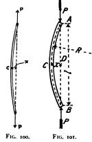
103. Limiting Load on Long Columns.—If, under the action of the load, the deviation x becomes greater, the bending-moment also becomes greater without any addition being made to the load; thus the deviation once started, may rapidly increase until fracture of the column takes place.
