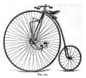
132. The Facile.-In the 'Facile' bicycle a smaller drivingwheel was used, and the mass-centre of the rider brought further behind the centre of the driving-wheel. This was accomplished
