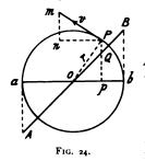
vibrating string, and of a particle of air in an organ-pipe when the simplest possible, is of this character. The speed of p will vary with its varying position. At any instant the velocity of the point P is in the direction P m, the tangent at P. Setting off v=Pm to scale along this line it may be resolved into two components Pn and nm respectively parallel, and at right angles, to ab. The parallel com-
