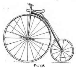
radial spokes only transmitted the weight from the hub to the rim. Figure 338 shows the 'Ariel' bicycle with a pair of lever tension wheels.
