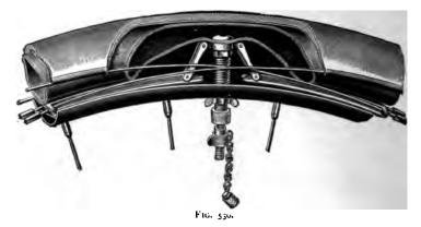
341. Devices for Preventing, and Minimising the Effect of, Punctures. - In the 'Silvertown Self-closure' tyre, which was of the single-tube variety, a semi-liquid solution of rubber was left on the inner surface of the tyre. When a small puncture was made, the internal pressure forced some of the solution into the hole, and the solvent evaporating, the puncture was automatically repaired.
