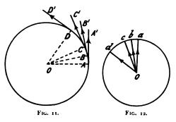
parallel to  $BB^1$ . Repeating this construction for a number of positions of the moving body, it is seen that the hodograph abc is a circle.
