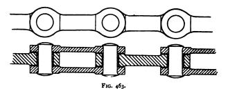
increased to one inch, giving a total pitch of two inches for the chain. If the side-plates be made to the same outline as the middle block (fig. 463), they may also be used to come in contact with the teeth of the chain-wheel. The chain-wheel would then
