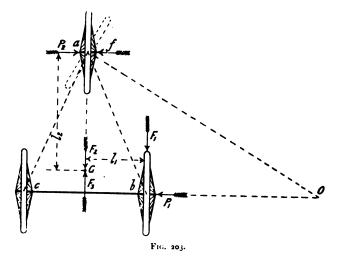
linear speed of the rim of wheel c will be greater than that of wheel b nearer the centre of rotation. If b and c are not drivingwheels, and are mounted independently on the axle, they will run automatically at the proper speeds. If b and c are driving-wheels, as in the 'Humber,' 'Cripper,' and 'Invincible' tricycles, some provision must be made to allow the wheel on the outside of the curve to travel faster than the inner. This is described in sections 188, 180.
