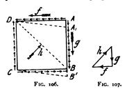
shearing stress on the planes A B and C D. If the planes A B and C D be very close to each other, the shearing stress will be the same on both. If q be the shearing stress per unit of arca, the downward force acting at A B and the upward force at C D
