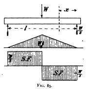
$\frac{W}{2}$ , the bending-moment at any section distant x from the end is therefore  $\frac{Wx}{2}$ , x being less than  $\frac{l}{2}$ . At the middle of the beam the bending-moment is a maximum, and equal to
