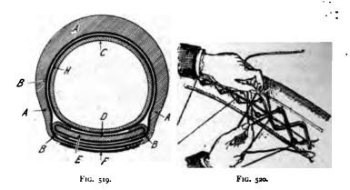
eight or ten inches. The outer-cover forms practically a tube slit for a few inches along its under side; this opening serves for the insertion of the air-tube, and is laced up when the air-tube is in place. When partially inflated the tyre is cemented on to the rim.
