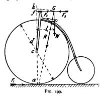
application of the brake to the front wheel, or by backpedalling in a Front-driver. (II) That in which the front wheel is quite free to revolve in its bearings; the header being caused by an obstruction on the road, application of the brake to the back wheel, or backpedalling in a Rear-driver.
