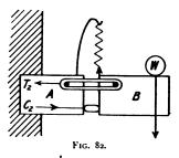
actually cutting the beam, and replacing by suitably disposed fastenings the molecular forces removed by the cutting. Figure  $8_2$  shows diagrammatically a cantilever treated in this manner. The shearing-force at the section is replaced by the upward pull IV of a spiral spring, and the couple acting on the part B formed by the load IV, and the
