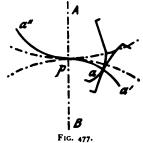
the pitch-line of wheel A will roll on the pitch-line of B. The angular speed of wheel A is now  $\frac{V}{r_1} + \frac{V}{r_2}$ . The instantaneous centre of rotation of wheel A is the point p, and therefore the linear speed of the point a on the wheel A is
