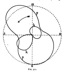
at giving the pedals a motion as nearly as possible like that of the foot during walking. PP (fig. 510) is the pedal path, p p (fig. 511) the polar curve of pedal speed, and k k the polar curve of speed of knee-joint, the dimensions of the mechanism being shown in figure 510. The construction is as shown in figure 498.
