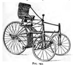
was much greater than in the 'German' tricycle (fig. 141). Another point of difference consisted in the application of the lever gearing; the pedals were fixed on oscillating levers, the motions of which were communicated by crank and connecting-rods to the driving-wheel.
