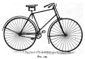
the crank-bracket, was usually curved, both in the diamond-frame and the cross-frame, or omitted altogether, as in the open-frame. Up till 1890 the nearest approach to the now universally adopted
