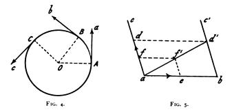
magnitude and direction, of the man is represented by the line  $a d^{1}$ . At the end of half a second the foot of the mast would be at *e*, *a e* being equal to  $\frac{1}{2} a b$ , and the man would have ascended the mast a distance a f; the actual position of the man would be  $f^{1}$ , midway between *a* and  $d^{1}$ . Thus his actual motion in space will be along the line  $a d^{1}$ .
