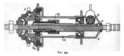
central pinion D can be locked. The intermediate pinions E, four in number, revolve on pins fastened to the hub  $C_1$  and  $C_2$ . The annular wheel  $G_2$ , which gears with the intermediate pinions, is made in one piece with the chain-wheel G. When the low gear is in use the central pinion D is held by the axle-clutch  $D_1$
