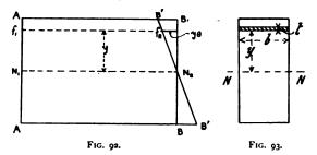
lines B and  $B^1$   $B^1$  gives the amount of the contraction or elongation of the corresponding fibres. The elongation or contraction of any fibre is thus seen to be proportional to its distance from NN. Now the stress on a bar or fibre is proportional to the extension produced; therefore the stress on the fibres of a beam varies as the distance from the neutral axis.
