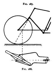
when turning a corner. The front fork would then be made straight, as it would act as a strut, while the stress would be almost entirely removed from the steering-tube.
