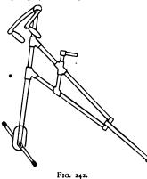
by the two straight tubes, each of which will be subject to bending-moment due to half the total weight.
