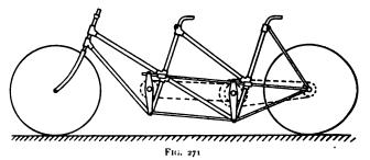
be pointed out that it is connected rigidly to the frame at four points, and may therefore be depended upon not to work loose.
