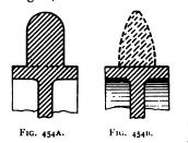
link is properly guided sideways on to the wheel. The cross section of the teeth is sometimes made as in figure 454A, the sides being parallel and the top corners rounded off. A much better form of section, which will allow of a considerable amount of swaying without danger, is that
