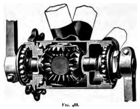
These hub gears, as far as we can see, have none of the advantages of the crank-axle gears to recommend them, since the speed of the chain cannot be increased unless a very large crank-
