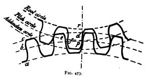
the tooth. The portion of the tooth outside the pitch-circle is called the *point*; and the portion inside, the *root*. The line joining the wheel centres is called the *line of centres*. The *top* and bottom clearance is the distance r d measured on the line of centres, between the addendum-circle of one wheel and the root-circle of the other. The *side-clearance* is the difference e f between the pitch and the sum of the thicknesses of the teeth of the two wheels, measured on the pitch-circle.
