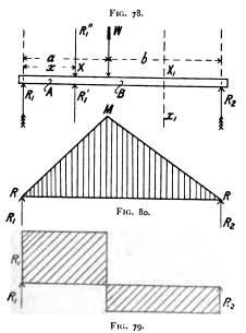
ing an ordinate of length equal to the shearingforce at the corresponding section, any convenient scale being chosen. The shaded figure (fig. 79) is the shearing-force diagram for a beam supported at the ends and loaded with a single weight.
