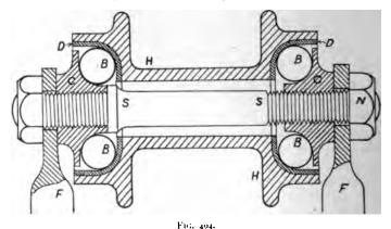
fork : hardened steel 'cones,' C C, are screwed on its ends, and hardened steel cups, D, are fixed into the ends of the hub, H, which is of softer metal. The balls, B, run freely between the cone C and the cup D. One of the cones C is screwed up tight against a shoulder of the spindle S, the other is screwed up until the wheel runs freely on the spindle without undue shake, it is then locked in position by a lock-nut N, which usually also serves to fasten the spindle to the fork end, F.
