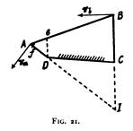
be the shortest, A B + D A be less than C D + B C, and A B - D Abe greater than C D - B C, D Awill rotate continuously, and C B oscillate. The speeds of points on the lever C B are proportional to their distances from the fixed centre of rotation C; similarly for points on the lever D A. Now in any position of the mechanism the link A B may
