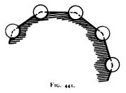
the chain-wheel might be made as in figure 441. With this ideal wheel there would be no rubbing of the chain-links on it as they moved into and out of gear.
