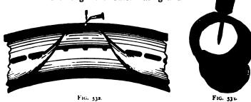
tread of the air-tube (fig. 533), and a small quantity of cement is left between the tread and the patching ply. On pressing down the tread the patching ply is cemented over the hole, and the tyre is ready for use as soon as the cement has hardened.
