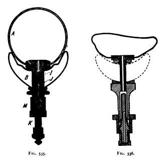
air in  $B^1$  is compressed until its pressure reaches that of the air in the tyre, the value V is lifted, and the air passes from  $B^1$ , along the hollow plunger, into the tyre. At the same time a partial vacuum is formed in the space B, and air passes into this space through the opening left between the plunger and the gland G.
