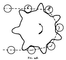
In a chain-wheel made with side-clearance, assuming the pitches of chain and teeth equal, there will be two pitch-polygons for the two directions of driving. Let a and b (fig. 447) be two consecutive corners of one of the pitch-polygons, and let the roller
