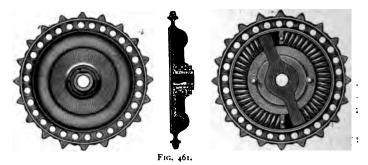
spring absorbs as soon as possible the variations of speed due to the chain-driving mechanism, and does not allow it to be transmitted to the pedals and the rider's feet.
