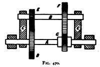
shaft B. The bearings of the shafts A and B are carried by the frame C. On the shaft B is fixed another wheel F, gearing with the wheel G, rotating loosely on the shaft A.
