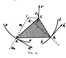
point on the curve a a; the corresponding position  $B_1$  is found by drawing an arc with centre  $A_1$  and radius A B, cutting the curve bb in  $B_1$ . With centres  $A_1$ and  $B_1$ , and radii A Cand B C respectively, draw two arcs intersecting at  $C_1$ . C will be a point on the path described by C.
