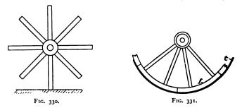
to bind the whole structure together. The compression wheel compares favourably in this respect with the tension wheel. On the other hand, the sectional area of the spokes must be great, in order to resist buckling under the compression ; very light wheels cannot, therefore, be made with compression spokes. The method of transmitting the load from the centre of the wheel to the ground is practically the same as in figure 330.
