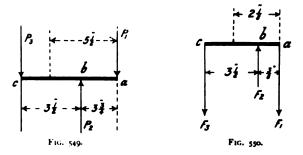
Consider now the horizontal forces. Fig. 550 represents the condition of affairs;  $F_1$ ,  $F_2$ ,  $F_3$  being respectively the horizontal L L 2
