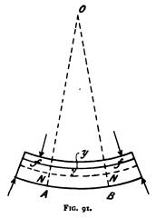
in figure 91. It can be easily seen that the bending-moment on the middle portion of the beam will be of the same value throughout, and if the section is uniform, the amount of bending will be the same at all sections; that is, the beam, originally straight, will be bent into a circular arc.
