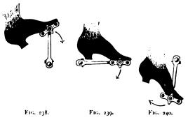
the arc of driving, ankle action has the further advantage of diminishing the extent of the motion of the leg. With a good ankle action the speed curves shown in figures 23, 501, and 511 may be considerably modified; in fact, the addition of a fifth link (between the foot and ankle) to the kinematic chain in figure 22 makes the motion of the leg indeterminate.
