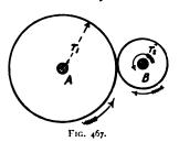
shafts A and B (fig. 467); if one shaft revolves it will drive the other, provided the frictional resistance at the point of contact of the rollers is great enough to prevent slipping. When there is no slipping, the linear speeds of two points, one on the circumference of each roller, must be the same. Let  $\omega_1$  and
