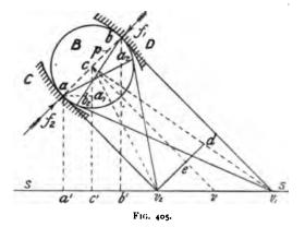
however, if a motion of rotation about the axis of the spindle, SS, be impressed on the whole system, equal in amount but opposite in direction to that of the centre of the balls round the axis, SS. The centre c of the ball B may thus be considered to be at rest, the ball to turn about an axis through its centre, the cup D and cone C to rotate in opposite directions about their common axis, SS.
