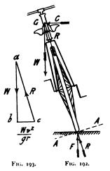
the ground, R. The resultant, C, of the two forces, W and R, must therefore be equal to the horizontal radial force
