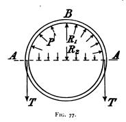
plane, A A, passing through the axis of the tube. The upper half, A B A, is under the action of the internal pressure p, distributed over its inner surface, and the forces T due to the pull of the lower part of the tube; therefore z T = the resultant of pressure p on the half tube. This resultant can be easily found by the following artifice : Consider a stiff flat plate joined
