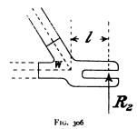
after being some time in use, and therefore some provision must be made for taking up the slack. This is usually done by making the distance between the centres of the crank-axle and the driving-wheel adjustable. Figure 306 shows a common faulty design for the stamping at the driving-wheel spindle. The force  $R_2$  (fig. 306) is equivalent to an equal
