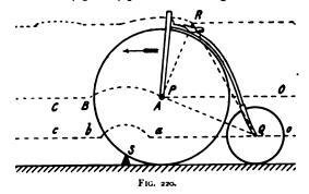
comes in contact with the obstacle at S, when the further motion of the wheel centre will be in a circular arc, AB, having S as centre. The further path of the wheel centre is the straight line, BC, parallel to the ground. The path of the centre of the rear wheel is of the same nature : a straight line, oa, until the tyre meets the obstacle S, the circular arc, ab, with S as centre, and then the straight line bc.
