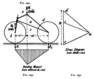
from the steering-head to the scat-lug is made stout enough to resist the bending-moment due to the saddle adjustment, while the seat-struts are subjected to pure compression, and the lower stays to pure tension. Figure 292 shows the stress-diagram for this braced structure; from which the thrust on the seat-struts, *a d*, is 116 lbs. If they are made of two tubes § in. diameter, 28 W.G., from Table IV., p. 112,  $A = 2 \times .0284 = .057$ , and the compressive stress is
