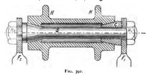
end of the spindle. If the bearing had worn loose, the cone C was screwed one or two turns further on the spindle until the shake was taken up. The cone was then locked in position by the nut  $n_1$ , which also fastened the end of the spindle to the fork. During this adjustment the other end of the spindle was held rigidly to the fork end  $F_2$ , by the nut  $n_2$ .
