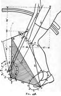
Produce H K to meet I P at J, then J is the instantaneous centre of rotation of the rider's leg K P from the knee to the pedal. From D and e draw dg and eg, meeting at g, respectively parallel to K H and P K. Since the points K and P are at the instant rotating about the centre J,
