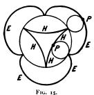
the fixed circle. The method of drawing these curves is similar to that of drawing the cycloid, the only difference being that the divisions along the path of the centre of the rolling circle will not be equal to those along the circumference of the rolling circle, but the divisions along the fixed and rolling circles will correspond.
