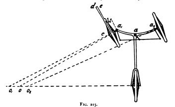
Cooper, the steering-wheels ran free on the same axle, which was pivoted at a to the rear-frame of the machine; the action in steering was therefore the same as in the 'Humber' tricycle. In
