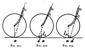
from the point of contact with the ground to the steering-axis, and  $l_4$  the half-length of the handle-bar.
