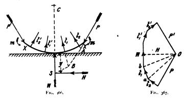
of a bicycle wheel. A general idea of the nature of the forces acting may be obtained from figure 366, which represents a small portion, XX, of the rim near the ground. This is acted on by the known force W; the upward reaction of the ground; by the un-
