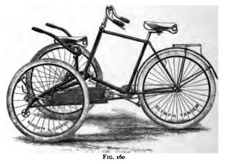
head placed as close as possible to the wheel, as in the 'Olympia' (fig. 160), one of the most successful of modern tricycles.
