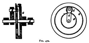
teeth in the wheel G fixed to the hub of the driving-wheel must then be 12 + 12 + 14 = 38. The driving-wheel of the bicycle is 46 in. diameter ; what is it geared to? Substituting in (7), the speed-ratio of the hub and the crank is  $\frac{52}{38}$ , and the bicycle is geared to  $\frac{52 \times 46}{38} = 62.95$  inches.
