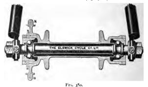
is screwed to the hub and the ball-races on the spindle are rigidly fixed. One important advantage of this form of hub is that the clear space which must always be preserved between the fixed spindle and the rotating hub is of much smaller radius than in the others. The area by which dust and grit may enter the bearing
