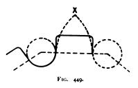
the roller and wheel is not along the circumference of the pitchpolygon; there is therefore a radial component tending to force the rollers out of the tooth spaces, that is, there is a tendency of the chain to mount the wheel (fig. 450).
