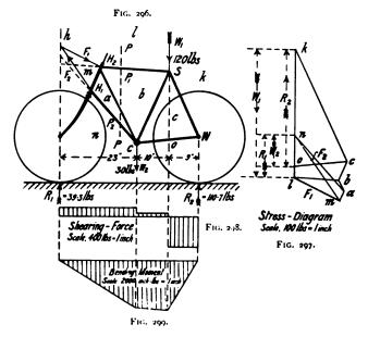
the reactions between it and the rear-frame, at  $H_1$  and  $H_2$ . These three forces must therefore (see sec. 45) pass through the same point. With the ordinary arrangement of ball-head the vertical pressure of the front portion of the frame acts on the rear
