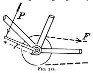
crank-axle, and chain-wheel. This rigid body is free to turn about the geometric axis of the crank-bracket, and it is acted on by three forces: P the pressure on the pedalpin, the pull F of the chain, and the reaction of the balls on the crank-axle. Taking moments about the geometric-
