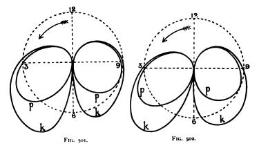
kept stiff during the motion. Using ankle action freely, the curve  $k \ k$  may not even approximately represent the actual speed of the knee; but the more rapid the variation of the radius-vectors to the curve  $k \ k$ , the greater will be the necessity for perfect ankle action. It should be noticed that with any mechanism a slight change in the position of the point H (fig. 497) may make a considerable change in the form of the curve  $k \ k$  (fig. 501).
