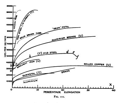
the extension being smaller, though the tenacity is very much greater, than that of mild steel.
