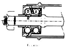
spindle run between coaxial cylindrical surfaces on the spindle and hub respectively; the motion of the balls, *B*, relative to both surfaces, is thus one of pure rolling. The space in which the balls run is a little longer, parallel to the axis of the spindle,
