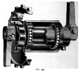
The arrangement of the two axles is shown diagrammatically in figure 492. When the high gear is in use the centre b of the crank-axle is locked in position vertically about the centre a of
